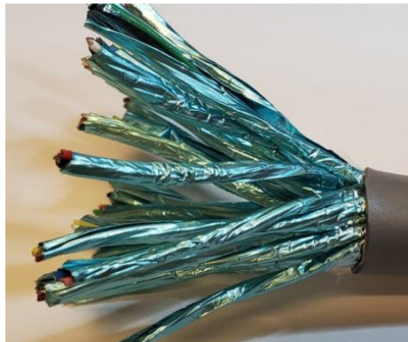
Pairs untwisted, first layer of shielding (clear) removed
